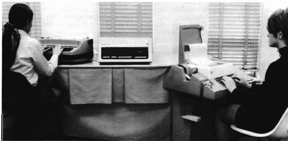
Wang 3300 BASIC uses either standard teletypewriters or modified IBM Selectric typewriters for input/output, accepts as many as 16 simultaneous users.
